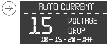
Picture 3. Automatic current regulation system
