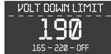
Picture 6. Low voltage protection
