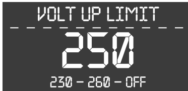
Picture 5. High voltage protection
