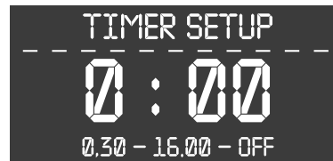
Picture 7. Delayed charging
